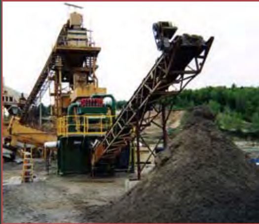
Palette Stone, NY - Recovered solids are conveyed to a stock pile where they are sold as product.
