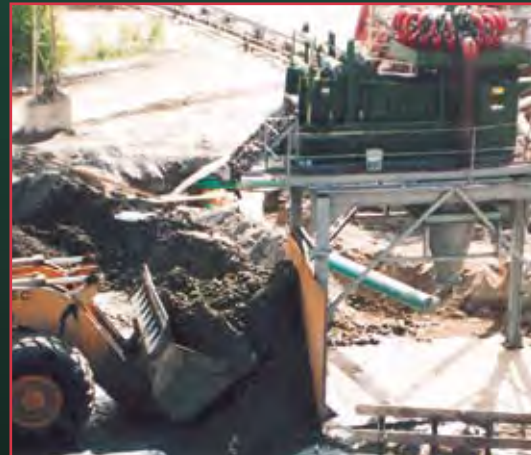
P.J. Keating Materials, MA - Recovered solids are more cost effectively handled with a pay-loader as opposed to drag lining solids or harvesting by excavator in a "soupy" form.
