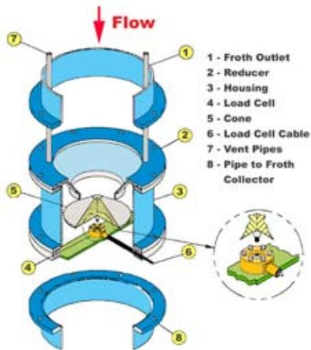
Patented Concentrate Mass Flow Measurement Device
