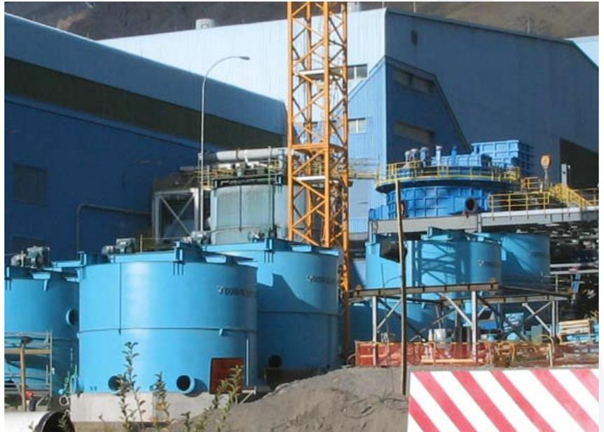
FLSmidth Dorr-Oliver Eimco pioneered the way for large cell technology. From its first Wemco 257m<sup>3</sup> cell installed in 2003, to now even bigger **300m<sup>3</sup> cells** being installed in Chile. These 26 x 300m<sup>3</sup> Wemco cells will be the first major installation of 300's for a new plant and the first used in rougher/scavenger duty!
