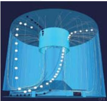
Computational fluid dynamic model of SmartCell® Flotation Machine operation.
