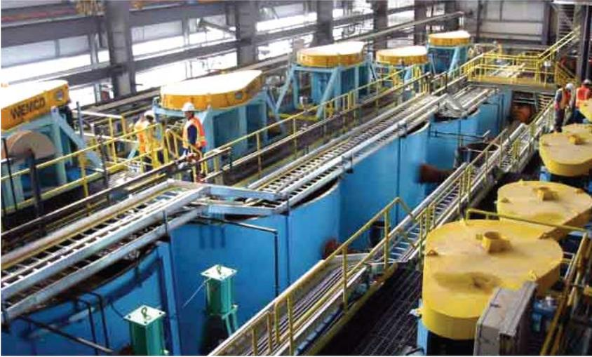
North American concentrator with 150 m<sup>3</sup> Wemco/Dorr Hybrid row. The Dorr-Oliver round tank cell includes many of the features developed for the world-leading Wemco® SmartCell® flotation machines.
