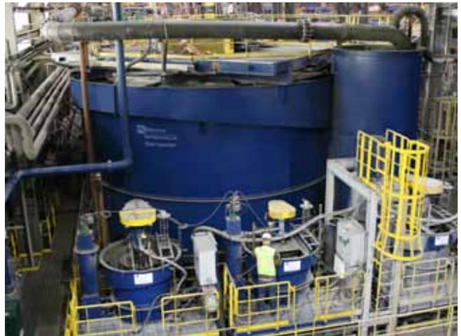
(Above) 350m<sup>3</sup> SuperCell installed with a Dorr-Oliver mechanism in a copper installation in the USA.
