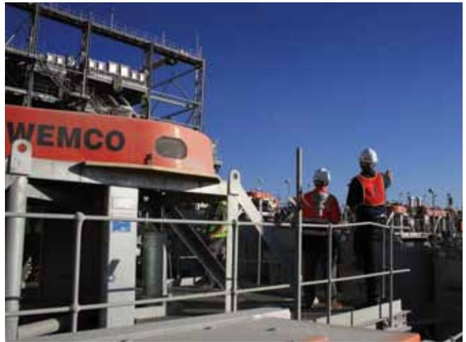
250m<sup>3</sup> Wemco Cells installed in a Copper plant in Mexico
