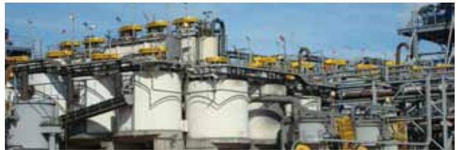
Below is a photo of the largest flotation installation in the world consisting of 66 250m<sup>3</sup> Wemco Flotation Machines located in Mexico
